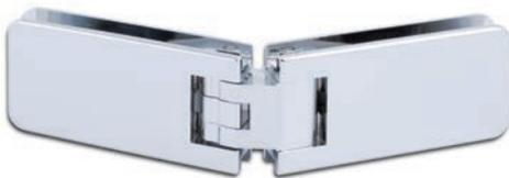
① Glass thickness 8, 10 mm · Self-closing from 15° · Continuously adjustable zero position · For mounting doors to a fixed sidelight
