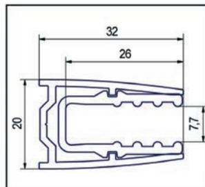
📌 Glass thickness 8 mm · Suitable for use with Aquant 40 sliding doors system · incl. plastic insert, no sealing required
