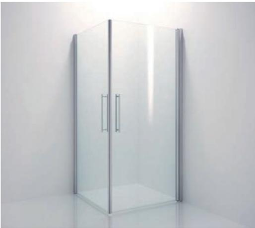
**i** Glass thickness 8 mm · Lifting height 5 mm · Hold position both sides at 90° · Profile length 2200 mm · Can be cut to the desired length · Please order two sets for double door applications. · Special profiles are also available as accessories for connecting to sidelights. · The deduction dimension of 13 mm has already been taken into account in the glass deduction for inserting the water deflector BO 5213494. If another water deflector is used, the deduction must be adapted accordingly.
