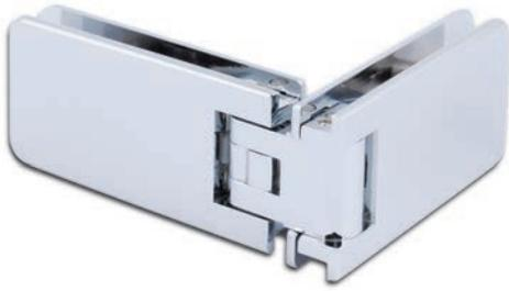
① Glass thickness 8, 10 mm · Self-closing from 15° · Continuously adjustable zero position · For mounting doors to a fixed sidelight
