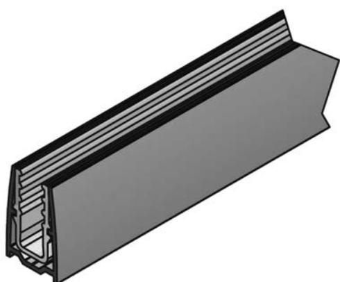
**i** Clamp-on profile for wall connection, suitable for use with Aquant 40 sliding doors system · Incl. plastic insert, no bonding/sealing required · Glass thickness 8 mm
