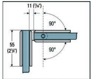
① Glass thickness 8, 10, 12 mm · Self-closing from 15° · Continuously adjustable zero position · For mounting doors to a fixed sidelight
