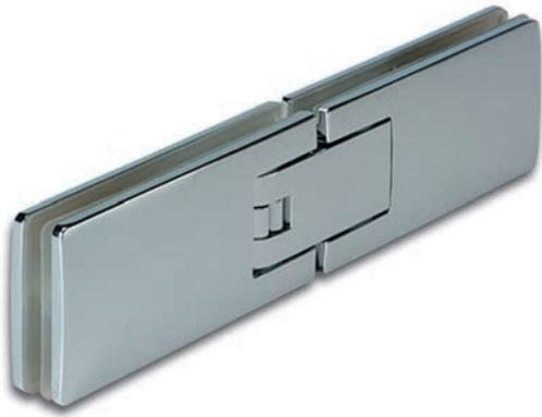
**i** Glass thickness 8, 10 mm · Zero position adjustable  $\pm 5^\circ$  · For mounting doors to a fixed sidelight
