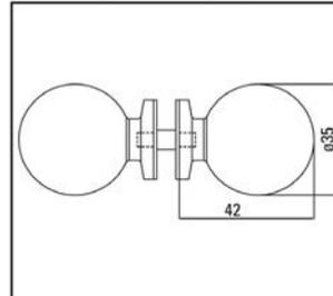
① Glass thickness tempered glass 6, 8, 10 mm · Drill hole in glass ø12 mm
