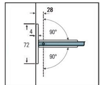
① Glass thickness 8, 10 mm · Zero position adjustable  $\pm 5^\circ$  · Supplied without mounting hardware
