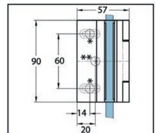
① The design of the groove enables the sealing strip to be simply guided through the hinge. Therefore, cutting the sealing strip or the bellow is no longer required. Glass thickness 6, 8 mm · Elongated hole for wall mounting · No glass cut-outs - only drilled holes are required
