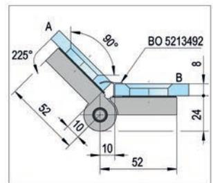
**i** Glass thickness 6, 8 mm · Lifting height 5 mm · The door is kept closed by magnetic seals.
