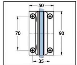
① Glass thickness 6, 8, 10 mm · Supplied without mounting hardware
