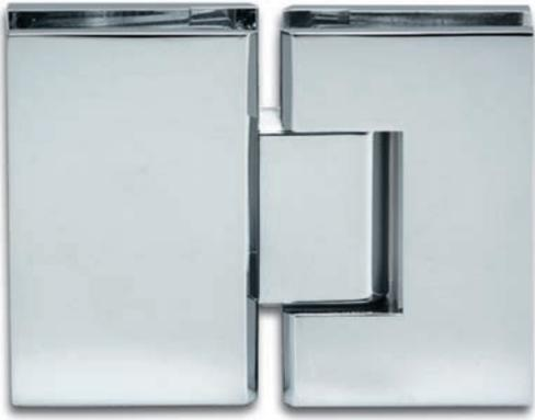
① Glass thickness 8, 10, 12 mm · Self-closing from 15° · For mounting doors to a fixed sidelight
