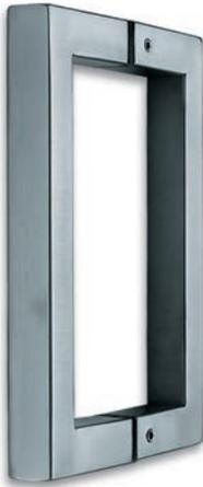
① Glass thickness tempered glass 6, 8, 10, 12 mm · Distance between centre drill holes (C-C) 152 mm · Drill hole in glass  $\varnothing$ 10 mm
