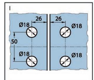
① Glass thickness 6, 8 mm · No glass cut-outs - only drilled holes are required
