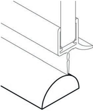
**i** Non self-adhesive · Threshold must be fixed individually and on site.
