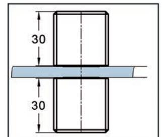
① Glass thickness tempered glass 8, 10 mm · Drill hole in glass ø12 mm
