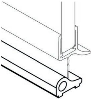
**i** Non self-adhesive · Threshold must be fixed individually and on site.
