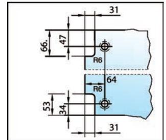
① Glass thickness 8 mm · Lifting height 5 mm · The deduction dimension of 13 mm has already been taken into account in the glass cut-out for inserting the water deflector BO 5213494. If another water deflector is used, the cut-out must be adapted accordingly.
