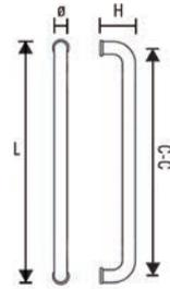
① Glass thickness tempered glass 6, 8, 10, 12 mm · Distance between centre drill holes (C-C) 375 mm · Drill hole in glass ø14 mm
