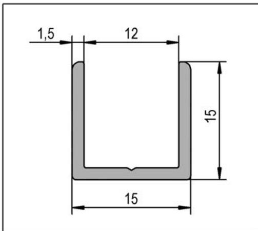
**1** Glass thickness 8 - 10 mm · Intended purpose: Installation of fixed partition walls, corner protectors, decorative cladding and a diverse range of other applications
