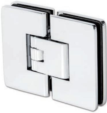
① Glass thickness 8 mm · Self-closing from 15° · Continuously adjustable zero position
