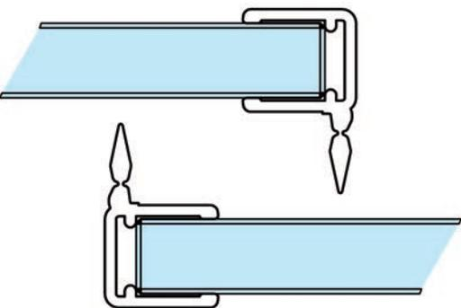
**i** Glass thickness 8 mm · sealing strips between fixed sidelight and sliding door · Packaging unit 1 pair
