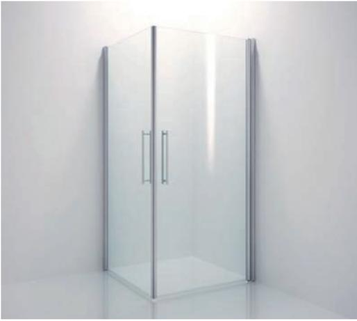
**i** Glass thickness 6 mm · Lifting height 5 mm · Hold position both sides at 90° · Profile length 2200 mm · Can be cut to the desired length · Please order two sets for double door applications. · Special profiles are also available as accessories for connecting to sidelights. · The deduction dimension of 13 mm has already been taken into account in the glass deduction for inserting the water deflector BO 5213494. If another water deflector is used, the deduction must be adapted accordingly.
