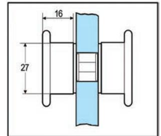
**i** Glass thickness tempered glass 6, 8, 10 mm · Drill hole in glass ∅16 mm
