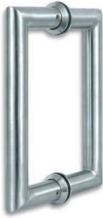
① Glass thickness tempered glass 6, 8, 10, 12 mm · Distance between centre drill holes (C-C) 203 mm · Drill hole in glass  $\varnothing$ 10 mm
