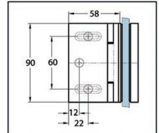
① Glass thickness 6, 8 mm · Elongated hole for wall mounting · No glass cut-outs - only drilled holes are required
