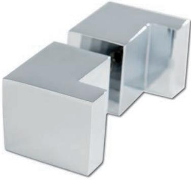
① Glass thickness tempered glass 6, 8, 10, 12 mm · Drill hole in glass  $\varnothing 10$  mm
