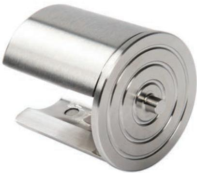
① Bonding plate for screwless floor mounting · with corrugated bottom surface for optimum distribution of the adhesive · only one stabilising bore hole in the floor needed
