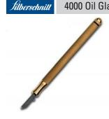
Brass handle with finger grips Cutting angle 138° · Straight edge stand-off distance 2.5 mm · Cutting head turns 30° · Narrow cutting head
