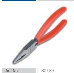
Plastic coated handles · ground head ideal for art glass work · small contact area  $\cdot$  little strength required  $\cdot$  less breaking risk Length 160 mm · Jaw width 4 mm
