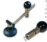
Trailing carbide wheel in Toplife quality improved break quality even for small radii · long service life · less cutting pressure Cutting angle 135° · minimum diameter 72 mm
