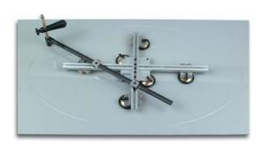
From 22 - 122 cm · for glass up to 25 mm thick using different wheel holders minimum diameter difference 6 cm · includes oil glass cutter 2000.S STANDARD 145°, T-handle, JOBO glass breaking device BO 705.0, cutting fluid, 2 felt-tip pens with adaptor · in practical aluminium case
