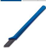
Toplife cutting wheel plastic handle can be placed underneath the score to break the glass · very light-weight cutting head made of special alloy · very fine, smooth cutting wheels not exchangeable glass cutting angle 138° · Straight edge stand-off distance 2.5 mm · for 2 - 6 mm glass
