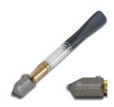
With replaceable, wide cutting head high-quality carbide cutting wheel · plastic handle with transparent oil reservoir · solid brass finger grip · traditional shape · The larger cutting wheel serves as a guiding aid when cutting with templates. Cutting angle 127° · Straight edge stand-off distance 2.5 mm
