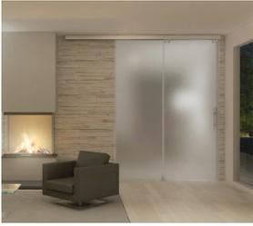
**i** Mounting Ceiling Mounting · Version double sided systems · Door weight max. 60 kg · Glass thickness sliding doors tempered glass 8, 10 mm · Glass thickness sliding doors laminated safety glass (made of tempered glass) 8.76; 10.76 mm
