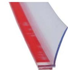
For sealing the shower door hinge side, length 2,200 mm, can be trimmed individually, for 8 mm glass, 16 mm lips, simple bonding onto the glass
