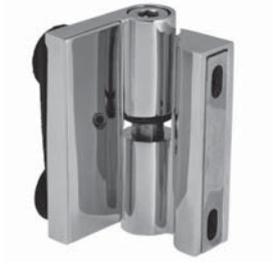
Rise and fall mechanism, flush receiving element, 2 drill holes required, for 8 mm glass, with screw BO 5200330, also 6 mm, wall fixation with dovetail guide
