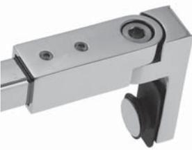
Glass clip for 8 mm glass, with screw BO 5200330, also 6 mm, drill holes required; angle freely adjustable, tube fixation with 2 grub screws
