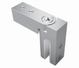
Glass clamp for 8 mm glass, with screw BO 5200330, also 6 mm, for clipping onto the glass; angle freely adjustable, tube fixation with 2 grub screws
