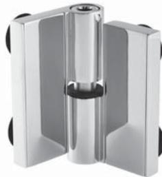
Rise and fall mechanism, flush receiving element, 2 x 2 drill holes required, for 8 mm glass, with screw BO 5200330, also 6 mm
