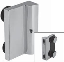
Corner connector for 8 mm glass, with screw BO 5200330, also 6 mm, for flush receiving element; drill hole required
