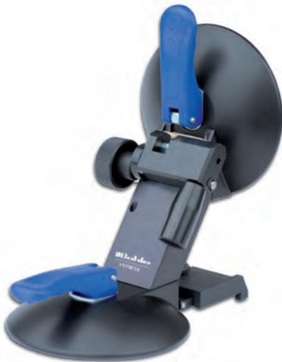
The Verifix® Pro angle suction holder is a high quality product topping the list of positioning and fixing devices for glass bonding. Especially in the case of UV bonds, as is common in glass furniture or showcase construction, Verifix® Pro offers superior protection against vibration and slipping - both for corner and T-joints. · Exact adjustment of the bonding gap (= thickness of adhesive layer) · extremely sturdy
