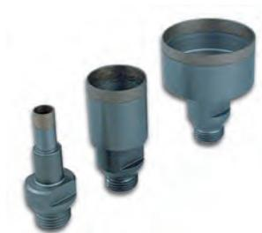
For normal use · drill base made of steel · covered with protective lacquer · diamond coating from sintered material · drill has to be sharpened before first use
