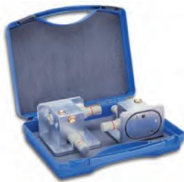
Verifix® pump-activated angle suction holder set in carrying case · as these positioning aids are mostly used in pairs, they are supplied as a set in a robust case ensuring that your valuable tools are well protected · the angle suction holders are also available separately. · A loss of vacuum is indicated by a red warning ring. The vacuum can be restored by simply pressing the hand pump.
