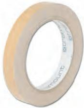
Xtramount® is a double-sided mirror adhesive tape made of closed-cell polyethylene foam (density 100 kg/m<sup>3</sup>), coated on both sides with a solvent-based, pure acrylate adhesive and protected on one side by blue silicone paper. Xtramount® was specially developed for vertical mounting of mirrors per DIN EN 1036, but can also be used for many
