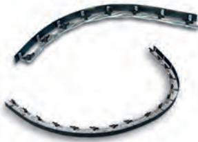
For cutting shapes in glass · ideal for the repair of arched glass doors and windows · suitable for inner and outer arcs · held in place with suction holder BO 670.5 (please order separately) · Recommended: three suction holders for 90 cm, six suction holders for 180 cm
