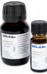
This activator allows the curing of Verifix® B 682-T UV adhesive where it is not possible under normal circumstances using UVA radiation, e.g. with coloured glass, screen printed glass, laminated safety glass, metal/metal bonds, etc. When activator is used, slight yellowing of the bond can occur. · Using an additional UV lamp is not required. · Shelf life: 6 months
