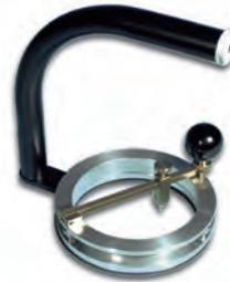
Ball-bearing · for small circles up to 9 cm ø · replaceable steel holder with Silberschnitt® carbide micro wheel for small radii
