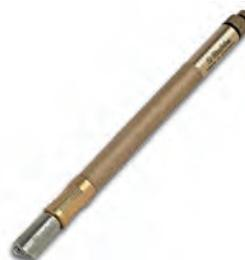
Perfect glass cutting · optimal application of cutting fluid ensures smooth glass breaking · 2-valve technology · round cutting head · trailing, exchangeable Toplife cutting wheels · sturdy brass handle · for shape and straight cutting
