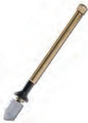
**i** Cutting angle 140° · Straight edge stand-off distance 2.5 mm · Glass thickness 3 - 12 mm · Cutting head turns 30°
