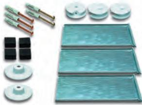
Press button set, for mirrors up to 2.6 m<sup>2</sup> · resting time only 30 minutes · suitable for humid environments and suitable to a limited extent for exterior applications · suitable for mirrors according to DIN EN 1036 · shelf life of 12 months from the date of delivery note
