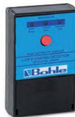
For detecting and determining the location of low-E coatings on single panes or double glazed units (4-10 mm glass thickness of individual panes). When checking double glazed units, measurements must be taken from both sides in order to determine the exact position of the coating.
