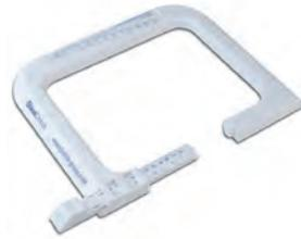
GlassCheck is used for measuring the overall glass thickness of already installed glass panes and insulated glass. The device is suitable for measuring glass thicknesses of up to 120 mm. The device also features an integrated glass thickness gauge which offers the possibility of determining the thickness of single glass panes (from 2 – 25 mm).
