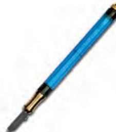
**i** Cutting angle 138° · Straight edge stand-off distance 2.5 mm · Glass thickness 3 - 10 mm · Cutting head turns 30° · Narrow cutting head
