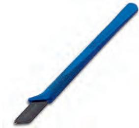
Glass cutter in Silberschnitt® 2000 quality · Toplife cutting wheel · plastic handle with traditional glazier's shape · can be placed underneath the score to break the glass · very lightweight cutting head made of special alloy · very fine, smooth cutting · an ideal all-purpose glass cutter · wheels not exchangeable
