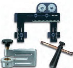
The combination of adjustable template, Silberschnitt® 2000 oil glass cutter with 360° revolving cutting head and cut opener makes lateral cut-outs possible · ideal for the production of toughened glass and shop fitting · includes case
