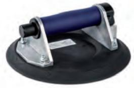
Pump-activated suction lifter made of sturdy aluminium with high load capacity for handling large objects. Handle with non-slip coating. The rounded pump tappet enables quick and easy operation and the red ring on the pump tappet enables permanent visual monitoring of the vacuum. The suction lifter is suitable for all materials with flat, airtight surfaces. The high quality of the suction lifter has been confirmed by TÜV (German Technical Inspection Agency) by granting it the GS sign.
