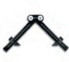
Plastic · with 2 suction pads for secure fixing · stoppers adjustable for corner or lateral cut-outs · infinitely adjustable · corner cut-outs adjustable from 45 to 400 mm, lateral cut-outs adjustable from 45 to 350 mm
