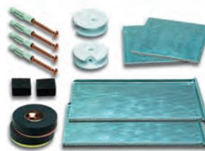
Magnetic set, for mirrors up to 1.6 m<sup>2</sup> · resting time only 30 minutes · suitable for humid environments and suitable to a limited extent for exterior applications · suitable for mirrors according to DIN EN 1036 · shelf life of 12 months from the date of delivery note
