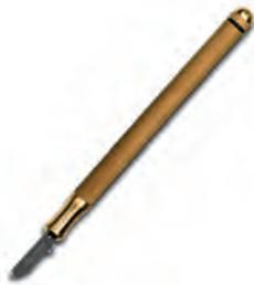
**i** Cutting angle 138° · Straight edge stand-off distance 2.5 mm · Glass thickness 3 - 10 mm · Cutting head turns 30° · Narrow cutting head
