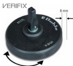
Eccentrically arranged, flat plastic disc · integrated suction pad · suitable for use when bonding floors or shelves in display cabinets · can be used individually or in pairs as precisely adjustable straight edge holder
