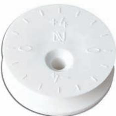
Eccentric discs are supplied with adjustment scale. The necessary height adjustment (+/- 4 mm = 8 mm) can immediately be read from the front of the disc. · With 5 mm  $\varnothing$  countersunk hole and lateral pinhole for easy adjustment. Made of high quality, impact resistant plastic.
