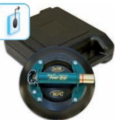
Powr-Grip® suction lifter for airtight materials. The lifter excels due to its greater carrying capacity (68 kg) compared to N4950 and a larger rubber pad (230 mm Ø). The flexible sealing lip is also suitable for handling curved surfaces. The red ring on the pump tappet warns the user in case of a significant loss of vacuum.
