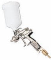
High quality starter model · Nozzle and needle made of stainless steel · Robust gun body made of extruded aluminium · Adjustable spray jet, material and air flow · For use with conventional compressed air lines · Complies with all relevant safety regulations · Practical and economical to use · Especially suitable for coating small batch runs · The gravity feed cup is ideally suited for use with BriteGuard® bottles (contents 500 ml)
