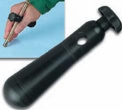
Ergonomic transverse handle for optimum application of higher cutting pressure · can be fitted to the metal models of Silberschnitt® oil glass cutters of the series 2000 and 5000 as well as BO 448.8 · individually adjustable to hand size
