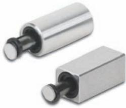
The pushbutton magnetic latches are suitable for glass doors or drawers whose fittings are not self-closing, i.e. without spring closing mechanisms. The magnetic latch must be positioned opposite the hinge (at the side where the door swings open). It does not matter whether the latch is placed closer to the top or to the bottom.
