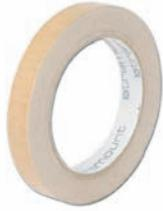
Suitable for concealed mirror rails BO 5208016 · Xtramount® is a double-sided mirror adhesive tape made of closed-cell polyethylene foam (density 100 kg/m<sup>3</sup>), coated on both sides with a solvent-based, pure acrylate adhesive and protected on one side by blue silicone paper. Xtramount® was specially developed for vertical mounting of mirrors per DIN EN 1036, but can also be used for many other materials such as metal plates, some plastics, glass or ceramic.
