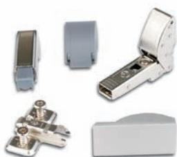
The Cristallo hinge in the glass/wood version can be combined with damper system or cover plate · new damping technology · for inset or overlay glass doors · snap on/off function · cross mounting plate for wood
