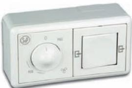
For infinitely adjustable speed control of ventilators · with switch for reversing air flow operation · on-wall mounting · overload protection by safety fuse · meets EC-RL 336/89-EC (EMV)
