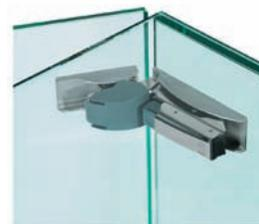
**i** Mounting glass/glass · Adjustment dimensions max. height / depth / width  $\pm 2 / 3 / 4$  mm · For inset and overlay doors · Opening angle 125 ° · For the load capacity, see image in kg
