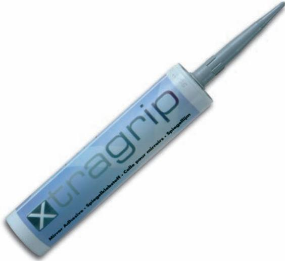
Solvent-free, neutral, silicone-based single-component adhesive (oxime-free). Intended for stress-compensating mirror bonding onto wood, concrete, stone, glass, metal, etc. Porous surfaces must first be treated with a primer. Not suitable for force-fit connections. Xtragrip® is easy to work with, stays permanently elastic, and does not corrode the mirror coating.
