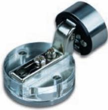
This attractive hinge with stainless steel bonding plate can be used for inset glass doors with two hinges. Adjustable in three dimensions. Equipped with a self-closing spring mechanism, it is ideal for use with the dampers BO 5500230/31 and BO 5500235/36.
