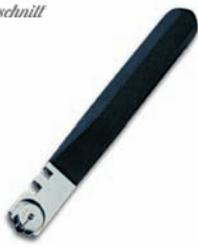
Ergonomic plastic handle especially for cutting tiles with strong pressure · replaceable, hardened turret with a carbide cutting wheel ø 5 mm
