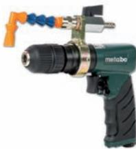
Metabo basic machine, retrofitted by Bohle for use as a water-cooled glass processing machine (order reduction nose BO 80.BG103 separately). For grinding tasks use in conjunction with abrasive diamond cartridges or other abrasive products. For grinding and polishing small drill holes, radii and breakouts with limited accessibility. Bohle offers an extensive range of corresponding supports and abrasive and polishing cartridges with graduated grits ranging from course grinding to fine polishing.
