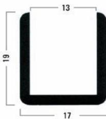
For installing fixed glass partitions · with radius corners · drilling guide in the bottom of the profile
