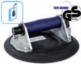
Pump-activated suction lifter made of sturdy aluminium with high load capacity for handling large objects. Handle with non-slip coating. The rounded pump tappet enables quick and easy operation and the red ring on the pump tappet enables permanent visual monitoring of the vacuum. The suction lifter lends itself to all materials with flat, airtight surfaces. The high quality of the suction lifter has been confirmed by TÜV (German Technical Inspection Agency) by granting it the GS sign.
