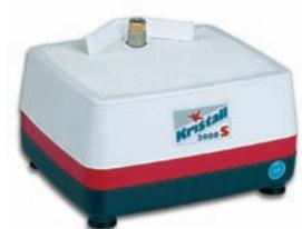
Glass grinding machine for all art glass work. The grinding head is cooled by an integrated pump which transports the coolant directly to the grinding head. Due to the efficient, double ball-bearing motor, the "Kristall 2000 S" can be additionally equipped, e.g. with the diamond band saw attachment TG H200. A 19 mm grinding head is included.
