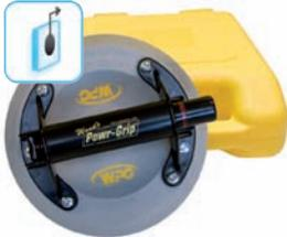
One of the new Powr-Grip® pump-activated suction lifters from the high quality N series. The lipped suction pad becomes attached quickly and easily to non-porous, flat surfaces. The special rubber blend of the suction pad prevents discolouring and stains on the surface. The red ring on the pump tappet warns the user in case of significant loss of vacuum.
