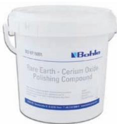
For removing small scratches or "blind" areas on glass in connection with a felt polishing wheel · mix polishing compound with water to form a paste and apply to glass surface · carefully polish with felt polishing wheel BO 5007901 · For straight line edgers and flat bevelling, manual and mechanical polishing
