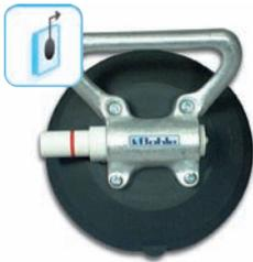
Suction lifter with sturdy metal handle · suitable for materials such as glass, plastic, metal, etc. · small curved suction pad, can also be used on surfaces with small radii · visual monitoring of the vacuum at the pump tappet
