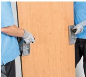
As a new feature, the Bohle Carry Clamp is now equipped with a rubber coating with diamond-shape texture. This coating helps prevent wet materials from slipping, particularly crafted stone or marble. The transported goods are held safely with two clamps - the heavier the load, the stronger the clamping mechanism.
