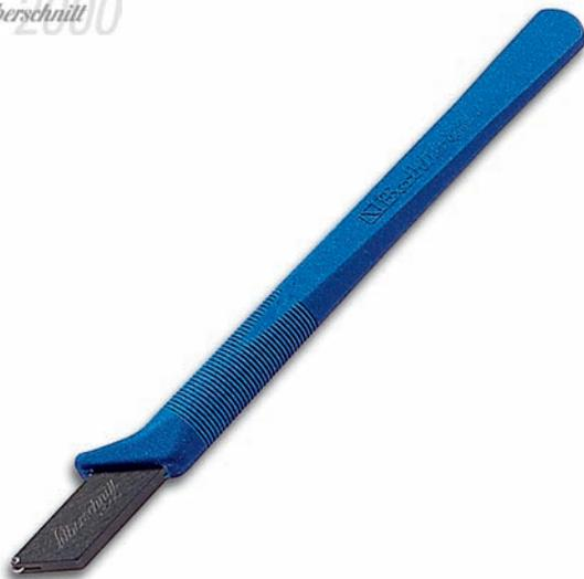
Glass cutter in Silberschnitt® 2000 quality · Toplife cutting wheel · plastic handle with traditional glazier's shape · can be placed underneath the score to break the glass · very lightweight cutting head made of special alloy · very fine, smooth cutting · an ideal all-purpose glass cutter · wheels not exchangeable
