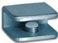
**i** Width Glass Shelf Support 30 mm · Glass thickness 6 - 10 mm · Projection maximum 160 mm · Width maximum 600 mm · Load capacity per pair max. 5 kg
