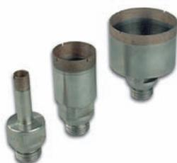
BO 5001402 with galvanic drill bit also suitable for LCD thin glass. Please set coolant water pressure at approx. 2.5 bar for reliable ejection of drill core.
