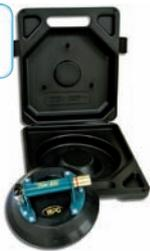
The Powr-Grip® pump-activated suction lifter with sturdy metal handle ensures a safe grip and lends itself for handling curved and airtight surfaces. The large curved rubber pad (250 mm Ø) makes this suction lifter especially suitable for curved glass panes. The red ring on the pump tappet enables permanent visual monitoring of the vacuum.
