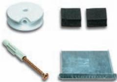
Mounting kit for mirrors up to 0.4 m<sup>2</sup> · resting time only 30 minutes · suitable for humid environments and suitable to a limited extent for exterior applications · suitable for mirrors according to DIN EN 1036 · shelf life of 12 months from the date of delivery note
