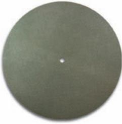
For disc grinding machines for wet grinding of glass parts · consists of flexible abrasive diamond coating and magnetic foil on the back · high flexibility: optimum attachment to the grinding discs · very long service life · high abrasive capacity · less heat at the grinding area
