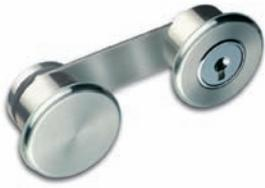
For UV bonding · stainless steel · universal key · bolt lock mechanism BO 5206259/58 is required · The lock is suitable for right and left handed doors as both bolt and lock cylinder can be turned around by loosening the screw.
