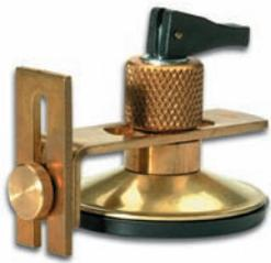
For multi-layered bonding, e.g. with two-component silicone adhesive. The adjustable holder is fastened by means of a suction pad to the corners of the glass panes. Rectangular glass sheets require a minimum of 3 units.
