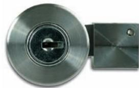
For UV bonding · stainless steel · universal key · please indicate glass thickness when ordering · The lock is suitable for right and left handed doors as both bolt and lock cylinder can be turned around by loosening the screw.
