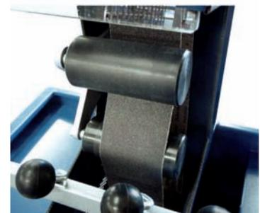
Belt position "lower edge grinding"
