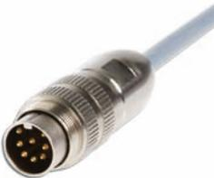
For connection of the digital inputs and outputs of the TinCheck® Industrial to an external application (e.g. control components) · with 8-pin IEC61076-2-106 connector one side, end open, length 10 m (other lengths on request)
