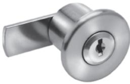
**i** Closing angle 180 ° · Drill hole in glass ø 25 mm · Material Lock nickel-plated · Sales unit 1 item
