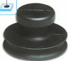
The Veribor® all-rubber suction lifter ideally lends itself to lifting and carrying different loads. It is suitable for holding smaller objects or for opening the covers of cable ducts. The vacuum is generated by simply pressing the suction pad onto the respective surface, which enables quick and efficient working. The lifter can be loosened from the surface by slightly lifting the release ridge.
