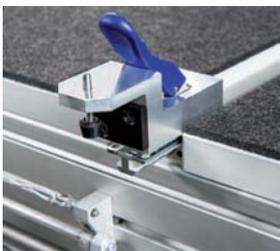
For fixing glass panes on the bonding table.
