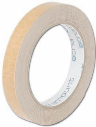
Xtramount® is a double-sided mirror adhesive tape made of closed-cell polyethylene foam (density 100 kg/m<sup>3</sup>), coated on both sides with a solvent-based, pure acrylate adhesive and protected on one side by blue silicone paper. Xtramount® was specially developed for vertical mounting of mirrors per DIN EN 1036, but can also be used for many other materials such as metal plates, some plastics, glass or ceramic.
