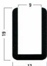
**i** Glass thickness 8 mm · Material Aluminium · Material thickness 2.0 mm
