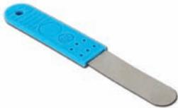
For use with the low viscosity UV adhesives B 665-0, LV740, LV740VIS, 420VIS. · When positioning the glass pane, a specific gap thickness can be adjusted with the aid of the thickness gauge. This guarantees that the minimum layer thickness of the adhesive is always observed. · Ideal for use together with the Verifix® Pro angle suction holders 90° (BO 639.0/ 639.1) and 45° (BO 639.2/ 639.3).
