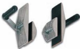
Suitable for transporting sheet materials · the load is held firmly between two non-slip, rubber-lined clamps · the heavier the load, the greater the clamping pressure
