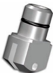
For optimised cutting, Bohle offers an additional model to the standard plastic wheel holders type 416. The cutting characteristics can be considerably improved due to the metal wheel holder BO 439.16 and the plastic rings which are colour-coded to indicate the different cutting angles. For shaped and open cuts the use of this type of wheel holder is recommended.
