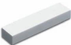
Removes used particles and creates a new cutting edge · after using the dressing stone, sharpen the drill with sharpening stone BO 5000499 · when drills are operated with little forward feed, no self-sharpening process takes place and the diamond particles turn blunt
