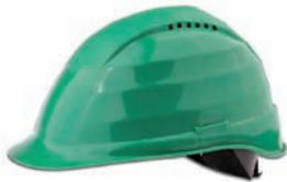
PE helmet · with rain catcher · plug-in holes for face/ear protection devices · side ventilation · four-point strap with sweat band · dimensional stability under heat: up to 70° C · breaking strength under cold: down to approx. -40°C · safety recommendation: not to be used for more than 5 years · do not use after heavy impact!
