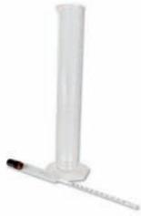
For determining the concentration of cerium powder in polishing liquid
