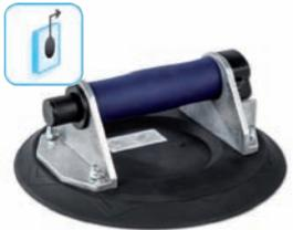
Pump-activated suction lifter made of sturdy aluminium for high loads. Handle with non-slip coating. The rounded pump tappet allows quicker and more convenient operation. The red ring on the pump tappet enables the permanent visual monitoring of the vacuum. The suction lifter is suitable for all materials with flat and airtight as well as slightly textured surfaces.
