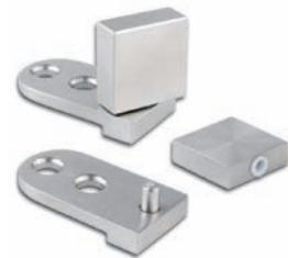
High quality stainless steel hinge suitable for inset doors · a threaded pin in the hinge enables the door to be removed after bonding
