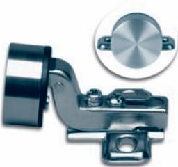
The well known Verifix® hinge is now also available in a glass/wood version · for inset doors · It can be adjusted in three dimensions and is equipped with a spring latch, ideal for use in combination with the dampers BO 5500230/31 and BO 5500235/36.
