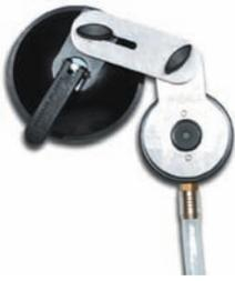
Precise drilling with little mess · the drilling dust is flushed with the coolant · a special sealing lip on the suction holder enables secure fixing even on relatively rough surfaces · special exchangeable drill bushings for 6, 8, 10 and 12 mm diameters · includes storage case
