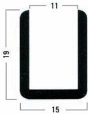
For installing fixed glass partitions · with radius corners · drilling guide in the bottom of the profile
