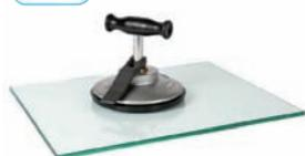
This suction lifter can lift almost any sheet material, no matter how textured its surface is. Due to its large, soft rubber pad, this Veribor® suction lifter ideally adapts itself to stone plates, chequer plates and structured floors. · Press the suction lifter with the T-handle firmly onto the surface and engage the large lever. As soon as you notice the resistance caused by generating the vacuum, the rubber pad adapts itself to the surface.
