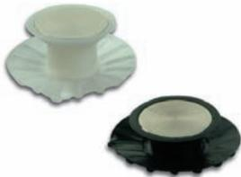
For flush mounting of mirror or glass elements indoors · incl. nickel-plated cover cap (stainless steel look) · minimum distance from glass edge to centre of drill hole: float glass and mirrors: min. 20 mm; tempered glass: 2 x glass thickness + 10 mm · Suitable fixing screw BO 5211153
