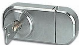
For UV bonding · universal key · stainless steel · suitable for all glass thicknesses · bolt lock mechanism BO 5206258/59 is required · can be retrofitted to finished objects or tempered glass door systems · The key can only be removed after locking.
