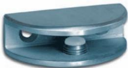
**i** Width Glass Shelf Support 50 mm · Glass thickness 6 - 10 mm · Projection maximum 200 mm · Width maximum 600 mm · Load capacity per pair max. 5 kg · Shape D-shaped
