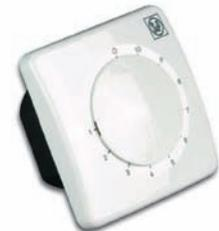
For infinitely adjustable speed control of ventilators · in-wall mounting · overload protection by safety fuse · meets EC-RL 336/89-EC (EMV) · unregulated switching output
