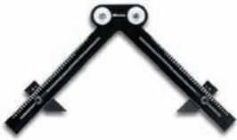
Plastic · with 2 suction pads for secure fixing · stoppers adjustable for corner or lateral cut-outs · infinitely adjustable · corner cut-outs adjustable from 45 to 400 mm, lateral cut-outs adjustable from 45 to 350 mm
