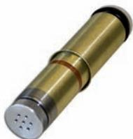
In general, all pump-activated suction lifters are equipped with a visual vacuum indicator at the pump tappet, i.e. additional pumping is required as soon as the red warning ring becomes visible, and visual control of the vacuum is ensured. This pump tappet has an acoustic vacuum indicator which issues a loud acoustic signal as soon as the vacuum diminishes.
