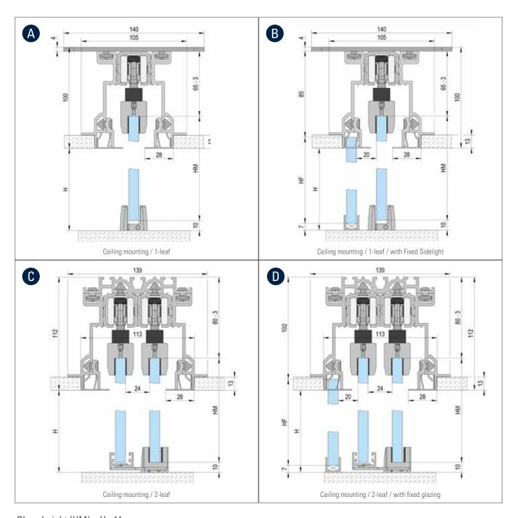
Glass height (HM) = H +11 mm Glass fixed part (HF) = H + 4 mm
