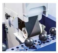
Belt position "lower edge grinding"
