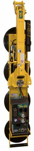
This vacuum lifter is designed to be particularly lightweight and space-saving. Thanks to its narrow dimensions, it is also ideal for applications that are especially difficult. Nevertheless, it can handle loads up to 320 kg. With manual 180° rotation and 90° tilt. Battery powered, it is equipped with a dual circuit vacuum system and can therefore also be used at construction sites.
