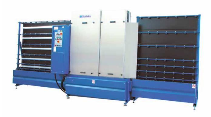
The powerful Bohle Verti-Clean glass washing machine is ideally suited for cleaning flat glass in the workshop or industrial applications. The automatic infeed forwards the glass into the washing area where it is thoroughly cleaned with four brushes.
