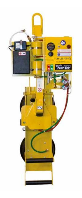
This vacuum lifter is designed to be particularly lightweight and space-saving. Thanks to its narrow dimensions, it is also ideal for applications that are especially difficult. Nevertheless, it can handle loads up to 135 kg. With manual 180° rotation and 90° tilt. Battery powered, it is equipped with a dual circuit vacuum system and can therefore also be used at construction sites.
