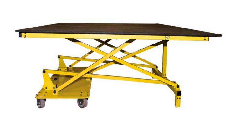
The Bohle Glazier's Tilting Table stands out due to its outstanding price/performance ratio and can be flexibly used as cutting table or workplace. The table is coated with high quality black felt.
