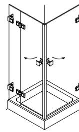
Pivot door on fixed glazing + pivot door on wall as corner application
