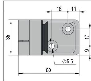
**i** Glass thickness 6, 8 mm · lifting height 5 mm · The door is kept closed by magnetic seals. Lugo shower door fittings must always be mounted together with sealing strips, which can be guided through the hinge. In order to avoid the incorrect operation of the door (opening against the opening direction), sealing strips and, if necessary, a stop should be used.
