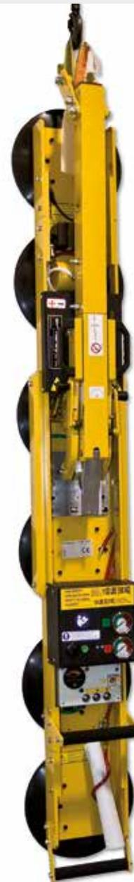
This vacuum lifter is designed to be particularly lightweight and space-saving. Thanks to its narrow dimensions, it is also ideal for applications that are especially difficult. Nevertheless, it can handle loads up to 500 kg. This lifter provides 180° rotation and 90° tilt. Battery powered, it is equipped with a dual circuit vacuum system and can therefore also be used at construction sites.
