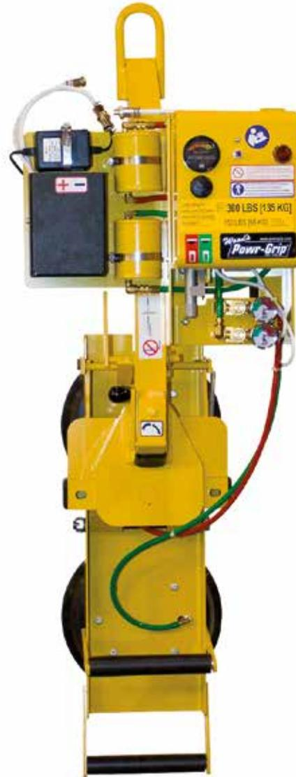
This vacuum lifter is designed to be particularly lightweight and space-saving. Thanks to its narrow dimensions, it is also ideal for applications that are especially difficult. Nevertheless, it can handle loads up to 135 kg. With manual 180° rotation and 90° tilt. Battery powered, it is equipped with a dual circuit vacuum system and can therefore also be used at construction sites.
