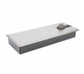
• Standard 10 mm plug-in flat conical floor spring axle included  $\cdot$  plug-in flat conical floor spring axle not exchangeable  $\cdot$  adjustable closing speed 90° - 15° / 15° - 0°  $\cdot$  ambient temperature -20° - +45°C  $\cdot$  tested over 500,000 cycles according to EN 1154  $\cdot$  dimensions 305 x 108 x 40.5 mm  $\cdot$  suitable for glass, wooden and aluminium doors
