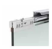
• Glass thickness door: toughened glass 8 - 12 mm, laminated safety glass 8.76 - 12.76 mm · no glass processing required · the running track is predrilled. · minimum door width 790 mm
