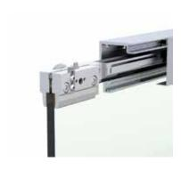
• Glass thickness door: toughened glass 8 - 12 mm, laminated safety glass 8.76 - 12.76 mm  $\cdot$  no glass processing required  $\cdot$  minimum door width 600 mm  $\cdot$  the running track is pre-drilled.
