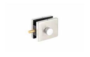
$\mbox{\Large 1}$  When used as a centre lock on double doors, one door must be used as a slave door.  $\cdot$  glass thickness toughened glass 10, 12 mm  $\cdot$  size 53 x 64 mm  $\cdot$  single throw / 17 mm bolt projection
