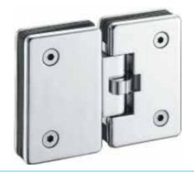
• Glass thickness toughened 8 - 12 mm, Hold open position 90°, Not suitable for one side opening, Door type - Swinging, Mounting - glass/glass 180°, max. door height - 2200 mm
