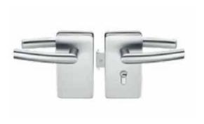
1 incl. profile cylinder with thumb turn, 4 keys and Keep for Double doors, single throw, 19 mm bolt projection, glass thickness toughened glass 10-12mm
