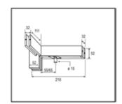
1 With pin ø15 mm  $\cdot$  adjustable pivot (55/65 mm)  $\cdot$  glass thickness toughened glass 10, 12 mm
