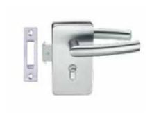
incl. profile cylinder with thumb turn, 4 keys and Stricker Plate for Single doors, single throw, 19 mm bolt projection, glass thickness toughened glass 10-12mm
