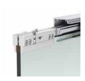
• Glass thickness door: toughened glass 8 - 12 mm, laminated safety glass 8.76 - 12.76 mm · no glass processing required · the running track is predrilled. · minimum door width 790 mm · please order cover caps separately if required.
