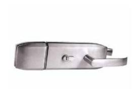
• incl. profile cylinder with thumb turn, 4 keys, Stricker Plate for Single door and Keep for Double door or to fixed sidelight, Nickel plated brass latch bolt, single throw, 19 mm bolt projection, glass thickness toughened glass 10-12mm
