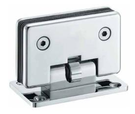
• Glass thickness toughened 8 - 12 mm, Hold open position 90°, Not suitable for one side opening, Door type - Swinging, Mounting - glass/glass 180°, max. door height - 2200 mm
