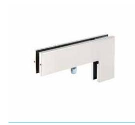
1 With pin ø15 mm  $\cdot$  adjustable pivot (55/65 mm)  $\cdot$  glass thickness toughened glass 10, 12 mm
