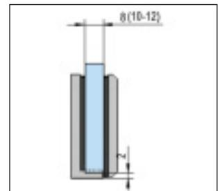
① Glass thickness 8, 10, 12 mm · Drill hole in glass  $\varnothing 18$  mm
