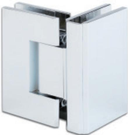
① Glass thickness 8, 10, 12 mm · Self-closing from 15° · Supplied with mounting hardware · For mounting doors to a fixed sidelight
