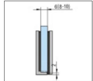
**i** Glass thickness 6, 8, 10 · Supplied with mounting hardware · For vertical partitions
