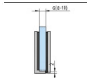
① Glass thickness 6, 8, 10 mm · Supplied with mounting hardware · For vertical partitions
