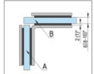
① Glass thickness 6, 8, 10 mm · Supplied with mounting hardware · For vertical partitions
