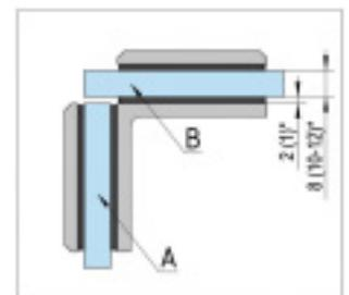
① Glass thickness 8, 10, 12 mm · Drill hole in glass ø18 mm
