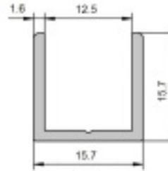
**i** Glass thickness 10 mm, Material Aluminium, Intended purpose: Installation of fixed partition walls, corner protectors, decorative cladding and a diverse range of other applications, Corrosion-resistant and therefore suitable for use in bathrooms and kitchens
