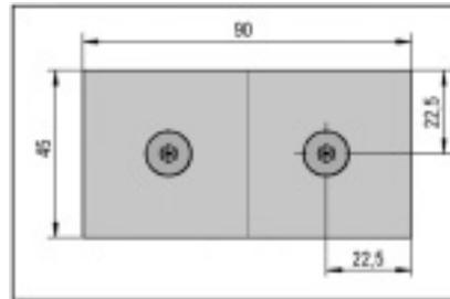
① Glass thickness 8, 10, 12 mm · Supplied with mounting hardware · For fixed partitions
