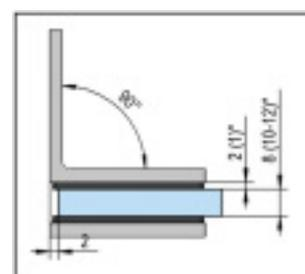
① Glass thickness 8, 10, 12 mm · Supplied with mounting hardware · For fixed partitions
