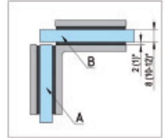
① Glass thickness 8, 10, 12 mm · Supplied with mounting hardware · For fixed partitions · x = glass thickness
