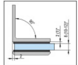
① Glass thickness 8, 10, 12 mm · Supplied with mounting hardware · For vertical partitions
