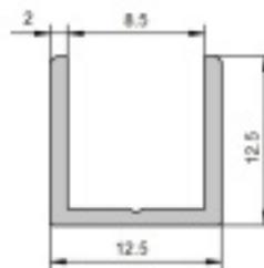
**i** Glass thickness 8 mm, Material Aluminium, Intended purpose: Installation of fixed partition walls, corner protectors, decorative cladding and a diverse range of other applications, Corrosion-resistant and therefore suitable for use in bathrooms and kitchens
