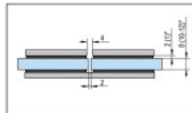
① Glass thickness 8, 10, 12 mm · Supplied with mounting hardware · For fixed partitions
