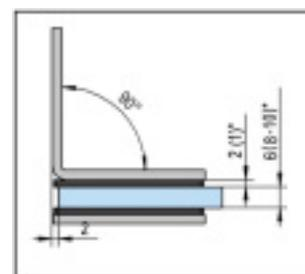
① Glass thickness 6, 8, 10 mm · Supplied with mounting hardware
