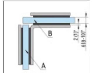
① Glass thickness 6, 8, 10 mm · Supplied with mounting hardware · For vertical partitions
