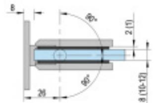
① Glass thickness 8, 10, 12 mm · Self-closing from 15° · Supplied with mounting hardware
