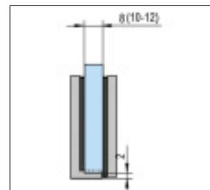
① Glass thickness 8, 10, 12 mm · Supplied with mounting hardware · For vertical partitions
