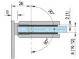
① Glass thickness 8, 10, 12 mm · Self-closing from 15° · Supplied with mounting hardware
