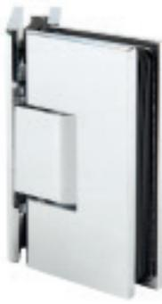
① Glass thickness 8, 10, 12 mm · Self-closing from 15° · Supplied with mounting hardware · For mounting doors to a fixed sidelight
