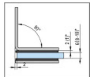
**i** Glass thickness 6, 8, 10 mm · Supplied with mounting hardware
