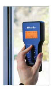
The Glass *Buddy*® from Bohle is the multi-talent for the accurate analysis of flat glass. This practical tool quickly and reliably supplies a multitude of information about the configuration of glass panes. In the past, similar glass analysis required many time-consuming measurements and calculations.
