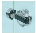
This hinge is a top quality stainless steel hinge for glass/glass mounting. Suitable for inset doors. It is adjustable in three dimensions and has a snapon function for easy mounting and dismounting. Equipped with a selfclosing spring mechanism, it is well suited for use with dampers BO 5500235/36.
